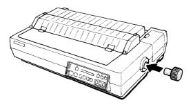
2. Press firmly on the knob until it fits against the printer case.
